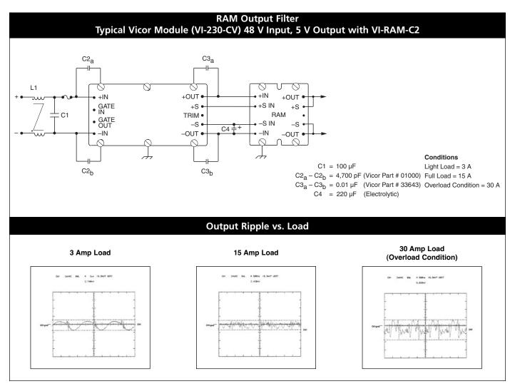
Figure 9–13 — Output noise, with Ripple Attenuator Module (RAM)
